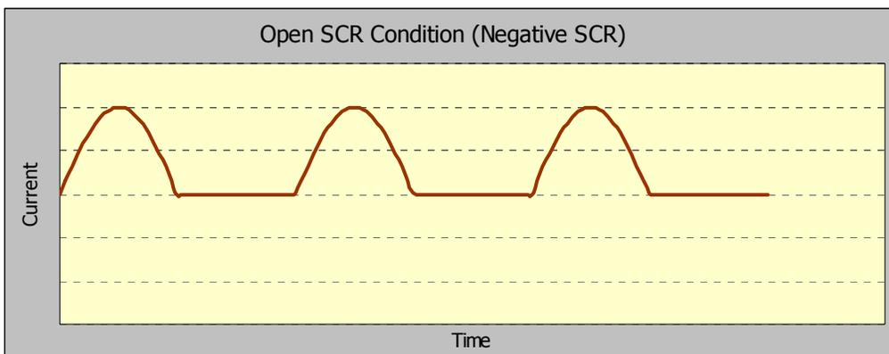
Figure 6: AC waveform through anti-parallel SCR pair with an Open SCR condition of the Negative SCR
