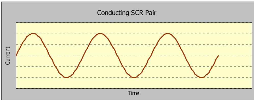
Figure 5: AC waveform through an anti-parallel SCR pair
