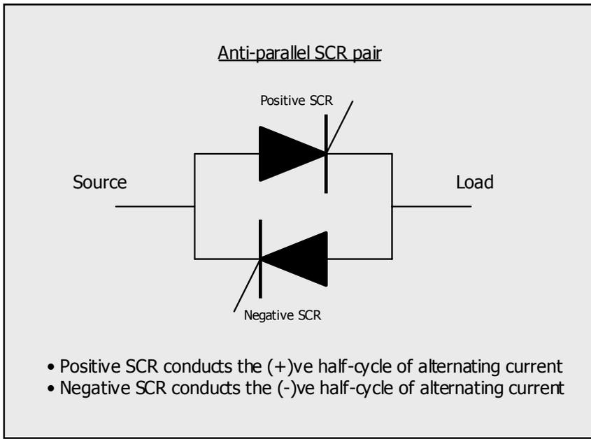
Figure 3: Anti-parallel SCR pair for AC waveform
