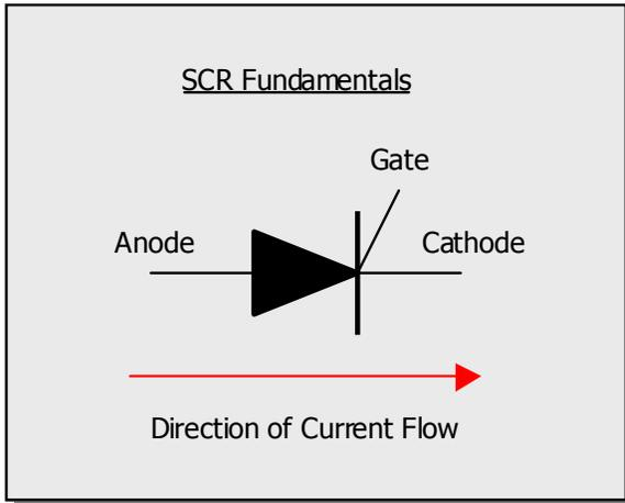
Figure 2: SCR Symbol and Flow of Current
