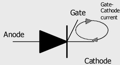
Gate-Cathode continuity is erroneously flagged as an healthy SCR on the inactive side
