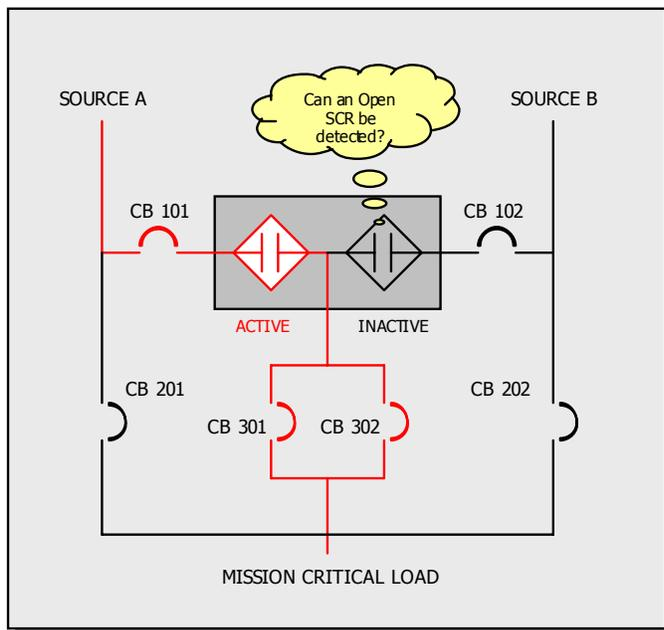
Figure 1: STS electrical one-line shows flow of power when Source A powers the critical load
