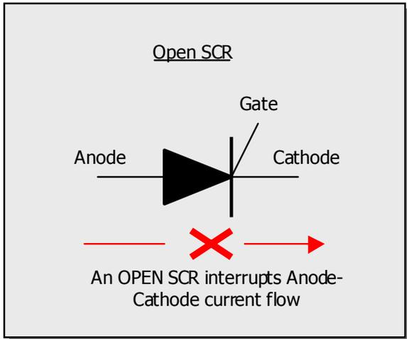
not possible to predict that a switch will close and conduct current (or will not close and will not conduct current when required) by observing the switch in its open state. In order to declare a switch defective, an attempt has to be made to allow it to carry current.
