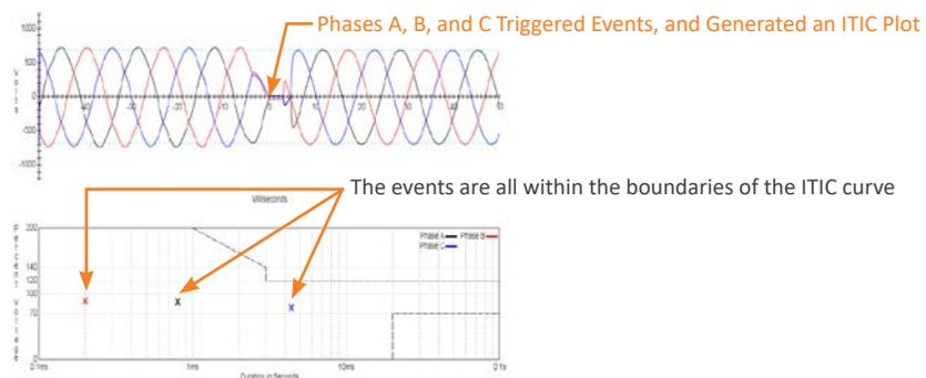
The ability to keep the transfers within the ITIC limits was verified through the Voltage Disturbance Analysis Tool (VDAT) plot shown above in the captured waveform.
