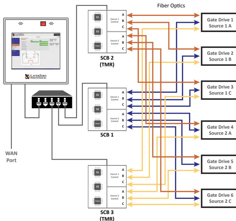
Reliability Features: Single Module Redundant (SMR) Redundancy
