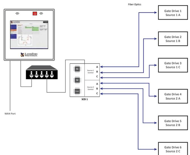
Reliability Features: Triple Modular Redundancy (TMR) \*Optional
