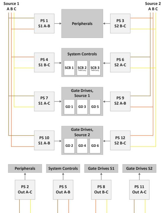
eSTS SMR Triple Redundant Processors
