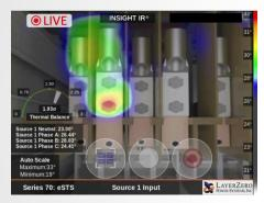
INSIGHT IR® uses a Network of Fixed-Mount Infrared Cameras to Capture and Record Temperatures Of All Customer Connections In Real-Time
